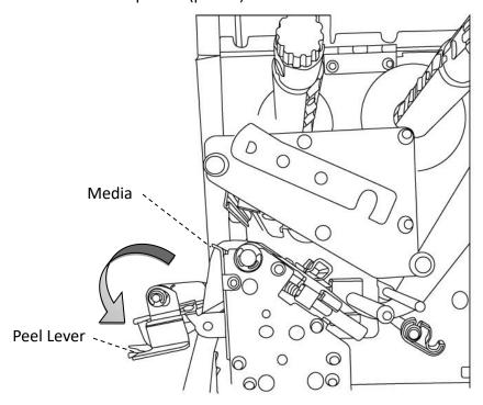
7. Close the dispenser (peeler) module using the peel-off mechanism release lever. Return the outside media guide and hook the head latch.
