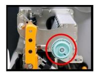
Step.2 Turn printer head rack clockwise to increase pressure or counterclockwise to decrease pressure.
