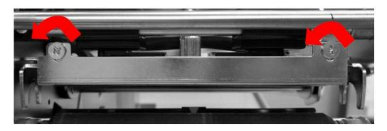
2. Make sure the Ribbon Bracket is at its **lowest** position first; then tight up the screws by rotating clockwise.
