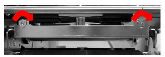
3. Alternatively, please reduce the occurrence of ribbon wrinkles through the ribbon wrinkle adjustment mechanism on both ends.
