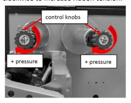
Too much tension at ribbon supply may result in ribbon not moving smoothly. Once it happens, rotate counterclockwise control knob of ribbon supply, to reduce ribbon tension to balance the tension.
