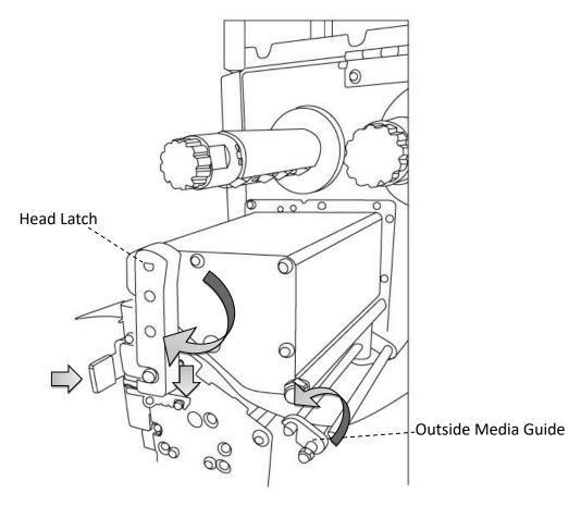
7. Close the top cover and turn on the printer or, press the FEED button if the printer is already on. The printer will then feed the labels through the cutter automatically.
