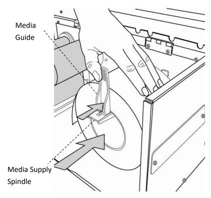
3. Rotate the head latch counterclockwise and open the outside media guide counterclockwise for media loading.
