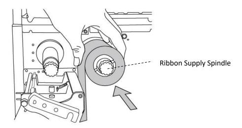
4 Thread the ribbon through the print head module. Place the edge of the ribbon on the bare core and wind a little onto the core. Make sure the coating side of the ribbon is facing down.
