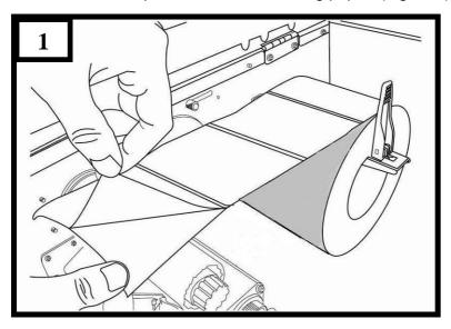
2. Lead the media backing paper through the print head module. (Figure 2)
