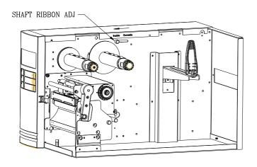
2. After the adjustment above, ribbon wound ink-side out can be used. Then install the ribbon:
