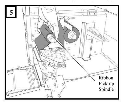
7. Turn the pick-up spindle to ensure the ribbon is tightly wound.
