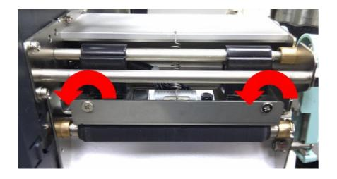
2. Make sure the Ribbon Bracket is at its lowest position first; then tight up the screws by rotating clockwise.
