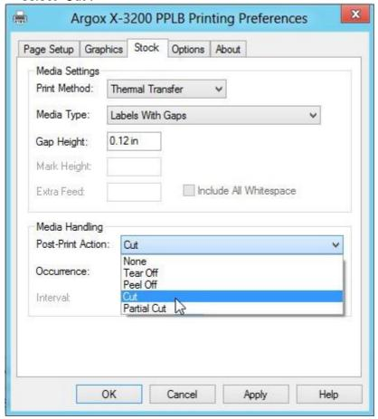
If there's Guillotine Cutter installed and partial cut function is needed, select "Partial Cut" in "Post-Print Action".
