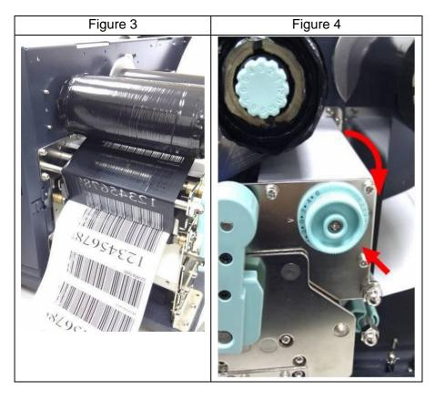
Once the desired quality has been reached, please make note on the new setting of the Fine Adjustment Knob and the type number of ribbon been used in this printing task for future reference.
