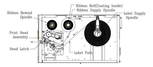
3. If ribbon wound ink-side in is in use, pull and move the <u>SHAFT RIBBON ADJ</u> to "Inside". Then install the ribbon:
