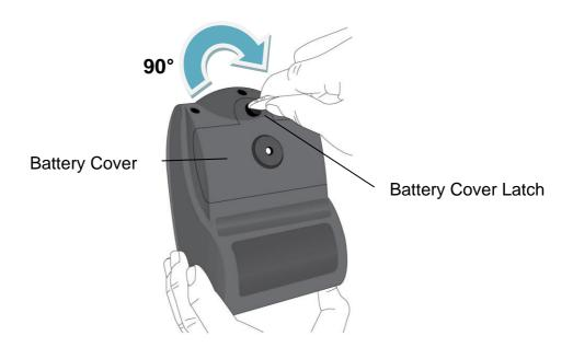
2. Remove the Battery Cover and install the Battery Pack into the
