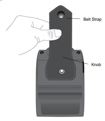
3. Insert the Screw onto the Knob, through the Belt Strap, and tighten clockwise until it is fully secured:
