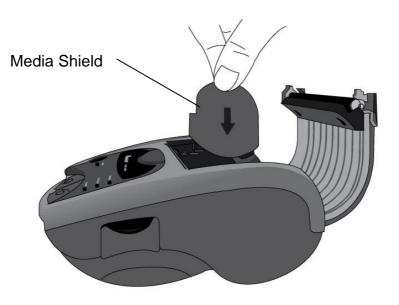
5. Pull a short length of media out of the printer. Close the Media Cover and press until you hear a click, to properly latch:
