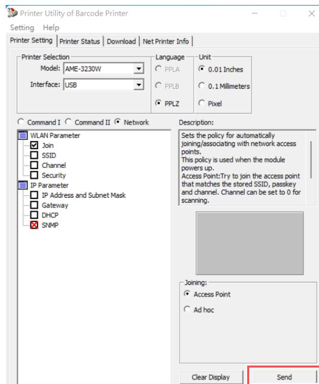
Please check the "SSID" box in the WLAN Parameter item. After checking the box, you can see the SSID input field at the lower right corner and enter the SSID of the Access Point you want to connect.
