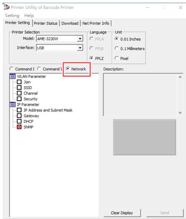
Please check the "Join" box in the WLAN Parameter item. After checking the box, you can see the Joining selection mode in the lower right corner and, for example, you can select "Access Point".
