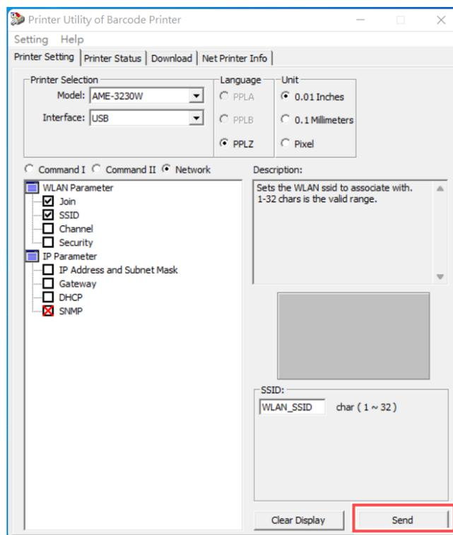
Please check the "Security" box in the WLAN Parameter item. After checking the box, select an encryption level to be performed and then enter the encryption key to be set according to the selected encryption level. When the two steps are complete, click Send.
