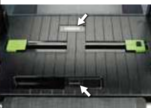
Twin-Eyed sensor system for paper detection
